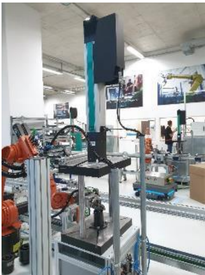
Image 4: Three of the automated press-in stations have TOX-2-Column Presses MBG, driven by a servo drive from the TOX-ElectricDrive series.
