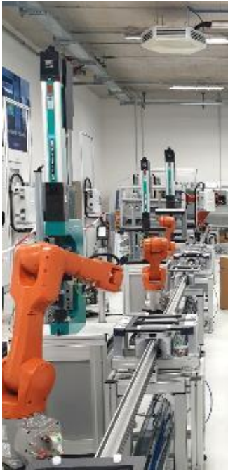
Image 3: Three of the TOX-Press-In Stations in the flexible assembly for Bonfiglioli gearboxes
