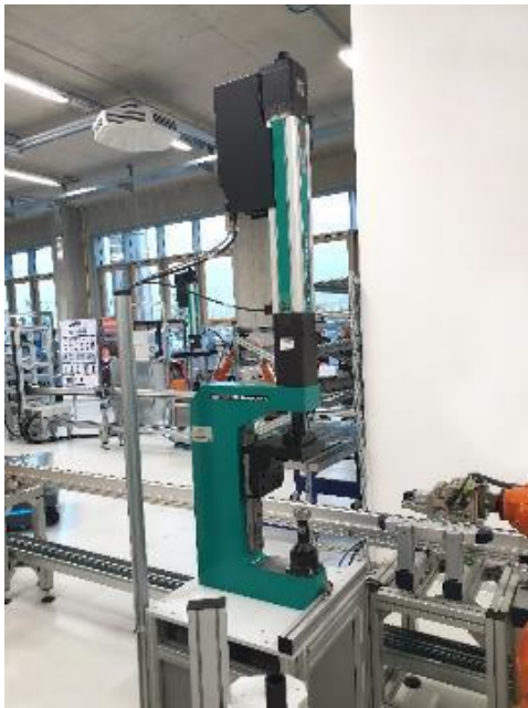
Image 5: The TOX-C-Frame bench presses can be perfectly integrated into the automated stations.
